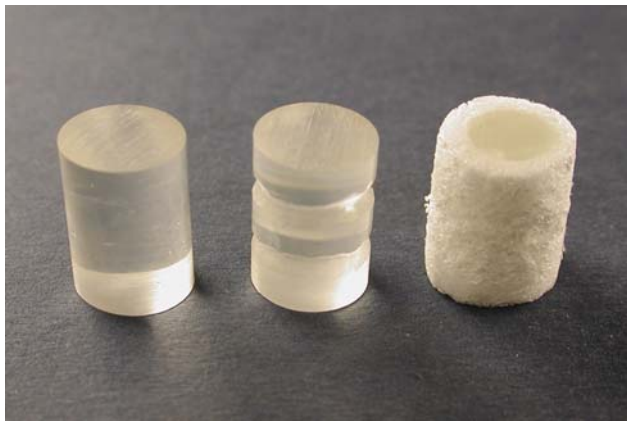
Figure 1 The test implants used in the push-out tests: (a) smooth surface (b) grooved surface and (c) porous surface. The implant with porous surface contained 10 wt% of chopped E-glass fibres and the IPF-process.
