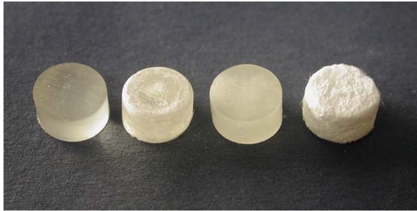
Figure 3 The implants used in HPLC residual monomer analysis: (a) 0 wt% of E-glass fibres, (b) 0 wt% of E-glass fibres, after the IPF process, (c) 10 wt% of chopped E-glass fibres and (d) 10 wt% of chopped E-glass fibres, after the IPF process.
